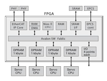
Fig. 5: FPGA configuration for 4-axes communication
